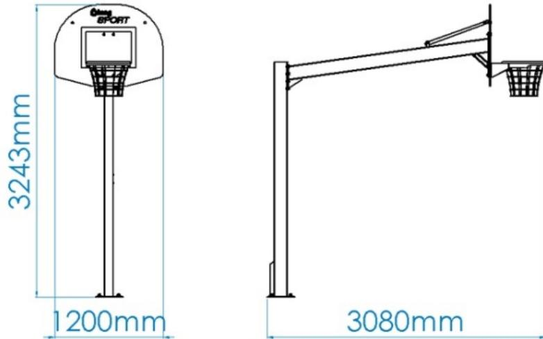
**INSTALAÇÃO / INSTALACIÓN / INSTALLATION / INSTALLATION**
